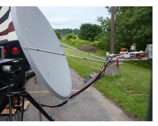
Heavy duty manual AZ-EL mount built by TerraCom that was originally used for portable point to point microwave link with a 4 ft fiberglass dish
